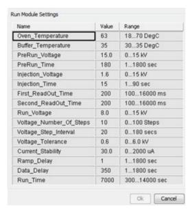
Figure 1. Optimized parameters for the 3730xl DNA sequencer.
