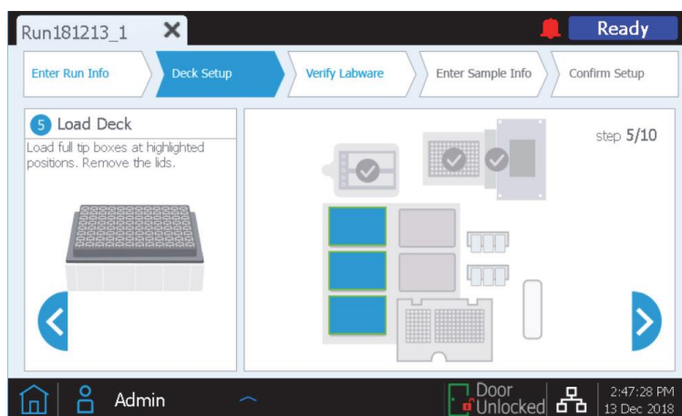
Figure 10. Step 5 of 10 of the Deck Setup screen of the Magnis NGS Prep instrument.
