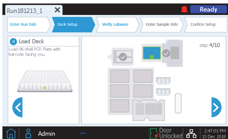
Figure 9. Step 4 of 10 of the Deck Setup screen of the Magnis NGS Prep instrument.
