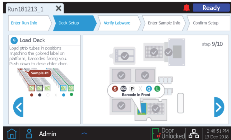
Figure 14. Step 9 of 10 of the Deck Setup screen of the Magnis NGS Prep instrument.
