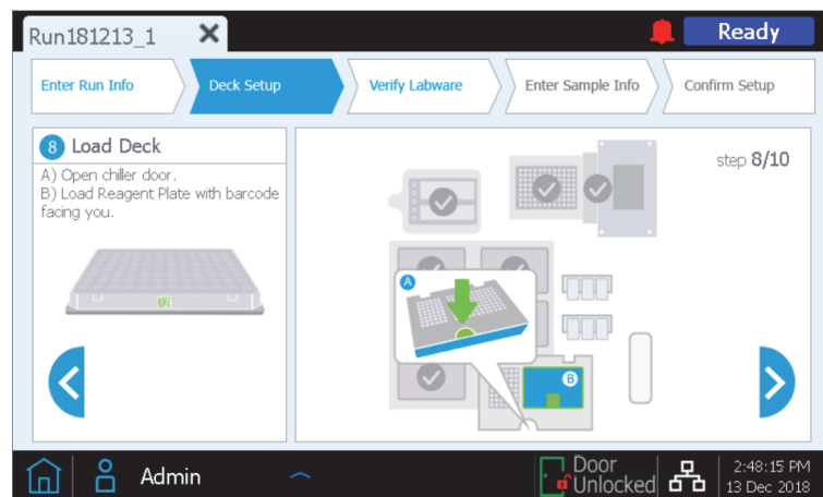
Figure 13. Step 8 of 10 of the Deck Setup screen of the Magnis NGS Prep equipment.
