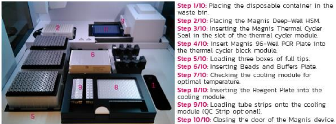
Figure 5. Magnis NGS Prep unit loaded for the assay and rapid load guide.
