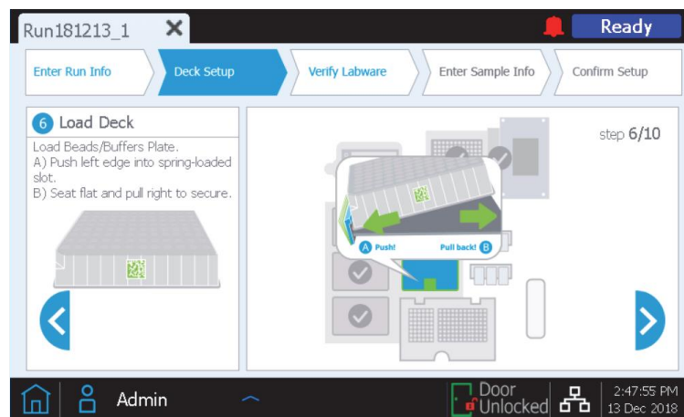
Figure 11. Step 6 of 10 of the Deck Setup screen of the Magnis NGS Prep equipment.
