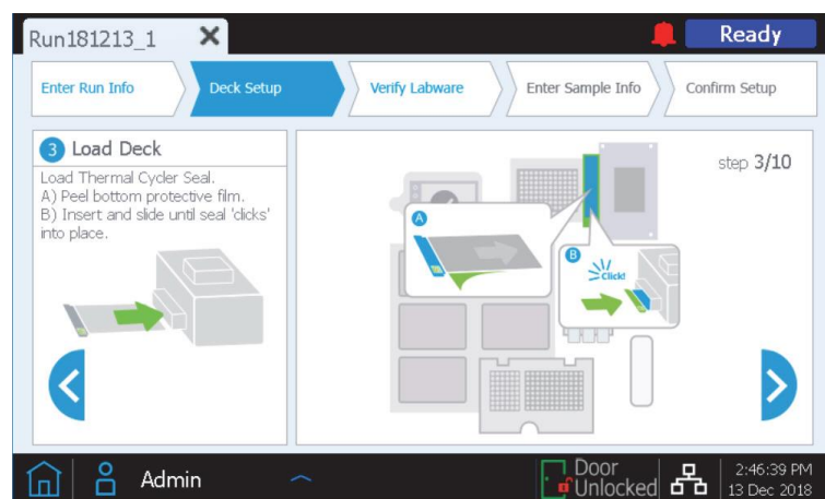
Figure 8. Step 3 of 10 of the Deck Setup screen of the Magnis NGS Prep equipment.
