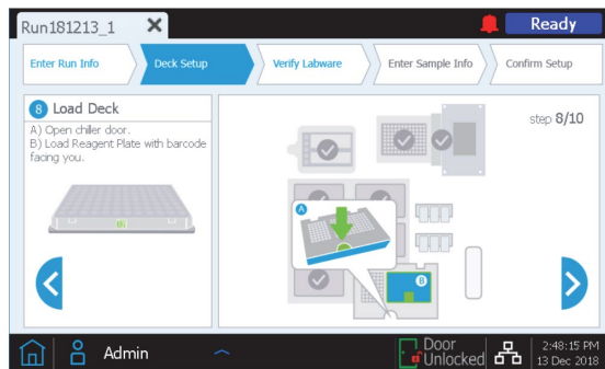
Figure 13. Step 8 of 10 of the Deck Setup screen of the Magnis NGS Prep instrument
