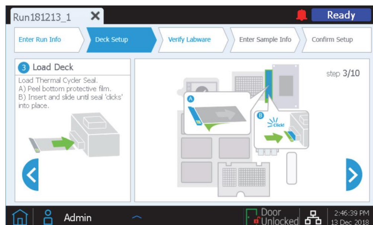
Figure 8. Step 3 of 10 of the Deck Setup screen of the Magnis NGS Prep instrument.
