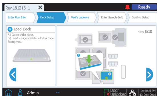
Figure 16. Step 8 of 10 of the Deck Setup screen of the Magnis NGS Prep instrument
