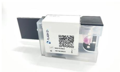
Figure 3. Left: Fully closed sample port lid is flush with the rest of the cartridge top.
