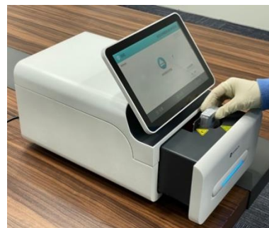
Figure 3. Left: Fully closed sample port lid is flush with the rest of the cartridge top.
