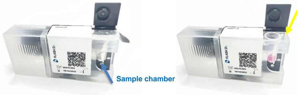
Figure 1. Left: Open cartridge showing the lyo pellet at the bottom of sample chamber; Right: Make sure that there is no foil left on the top of sample chamber.
