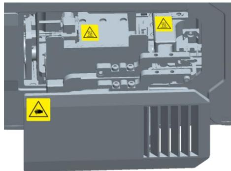
**Fig.1-4 Labels On The Heating Module**
