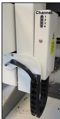
Figure 7: Pipetting arm with pressure monitoring system.
