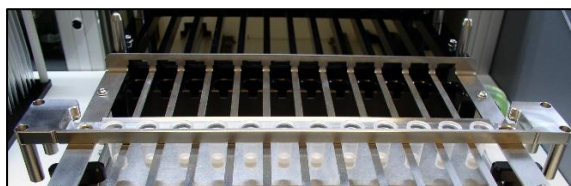
Figure 17: Loading position for the column rack on the empty Buffer cartridge rack.
