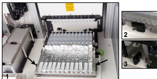
Figure 25: Loading procedure of the filled buffer rack into the instrument. The rack is fixed on both sides by black clips (black arrows, part 1). Clip open (part 2) and clip closed (part 3).
