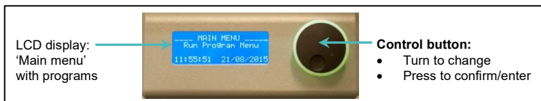
Figure 6: Control panel with Control button of the instrument.
